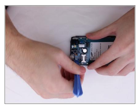
Use the flat end of a spudger to disconnect the camera assembly cable.
