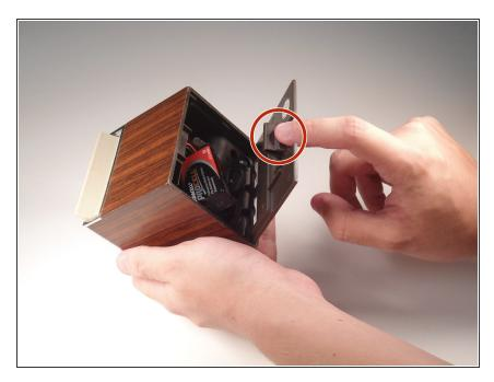
To remove the back panel from the Weather radio, use your index finger and push down on the tab located on the back.
