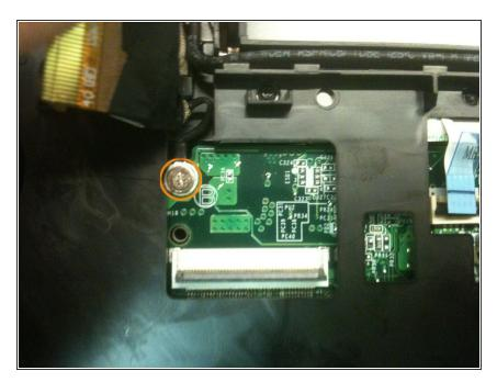
Unscrew the ground screw pictured here. It will remain attached to its cable via a retaining clip.
