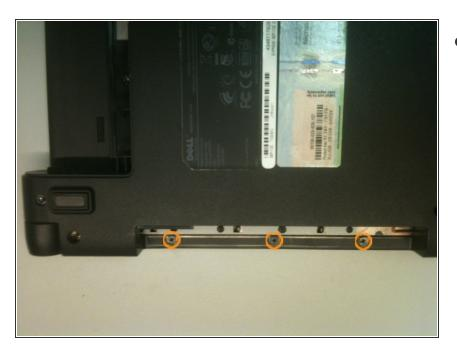
Remove 3 small (2.5x3mm) screws from the optical drive bay area.
