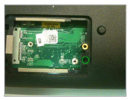
Remove one long (2.5x5mm) screw from the accessory bay. NOTE: In some versions of the laptop, this screw is not accessible or may not exist. If that is the case, you can ignore this step.
