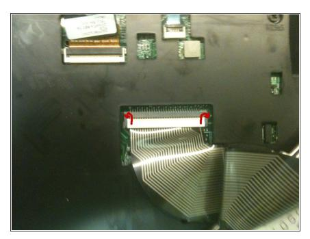
Remove the keyboard cable from the motherboard in the same way you removed the 'PB' cable from step 8, and set the keyboard aside.
