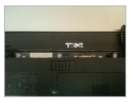
Slide the battery lock switch to 'unlock' position and remove battery to reveal three silver phillips screws (5mm length). Remove these.
