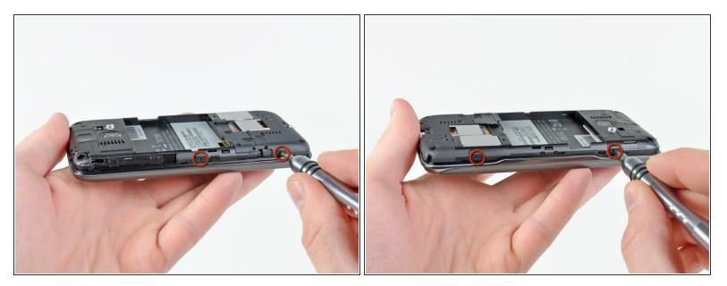
Four more Phillips screws along the edges of the phone secure the rear case to the body of the HTC Surround.
