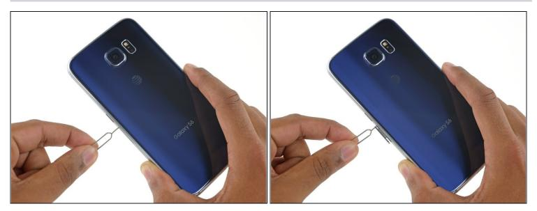
• Insert a paper clip or SIM eject tool into the hole in the SIM card slot on the power button side of the phone.
