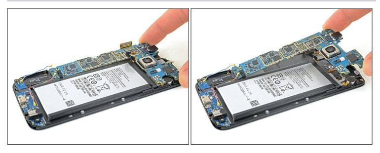
Lift the camera-side end of the motherboard to separate it from the display frame.
