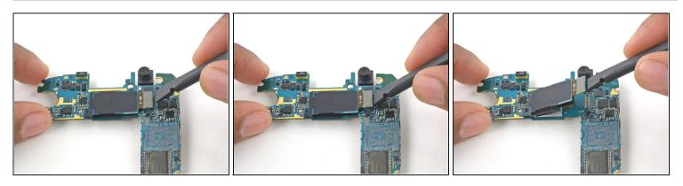
• Use the flat end of a spudger to disconnect the rear-facing camera connector from its socket on the motherboard.
