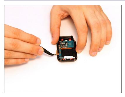
• Using a pair of precision tweezers, gently grip and disconnect the AMOLED display connector from the mainboard.
