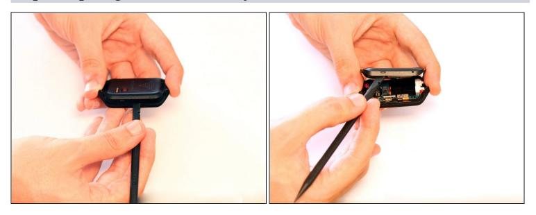
• Once the four Torx screws have been removed from the Watch Assembly, using a spudger, gently pry the front and back halves of the watch away from each other. This is best accomplished by placing the head of the spudger in the space between the two halves and rotating the head until the two halves split apart.
