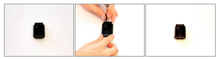
• Start by removing the four Torx T5 Security Screws from the back panel of the Watch Assembly.
