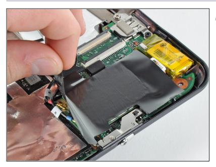
(i) If present, carefully peel the piece of tape covering the WWAN board.
