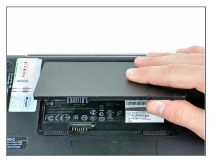
• Lift the battery out of the Mini 1000 from the edge closest to the release latches.
