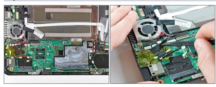
*i* If present, remove the pieces of black cloth tape securing the antenna cables to the motherboard.
