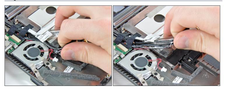
• Carefully untangle the fan cable from the bundle of cables leading to the display.
