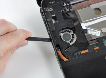
Repeat the same procedure as mentioned in the previous step to release the clips along the left side of the upper case.
