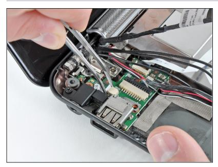
Use a pair of tweezers to pull the internal display switch cable straight away from its socket on the USB and power board.
