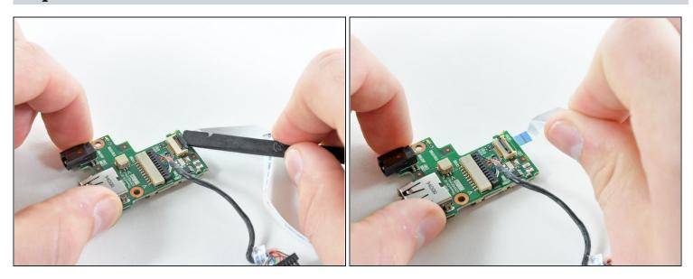
• Use your fingernail or the flat end of a spudger to flip up the retaining flap on the SIM card cable ZIF socket.
