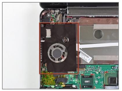
i If present, remove the large piece of black adhesive film covering the area around the fan.
