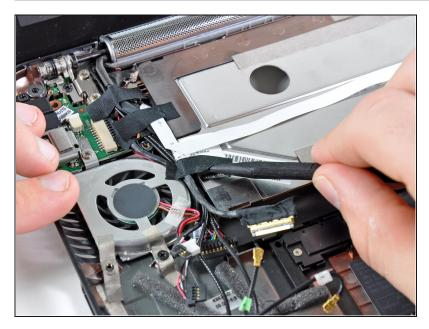
(i) If present, remove the piece of black cloth tape holding the bundle of cables to the top of the fan.
