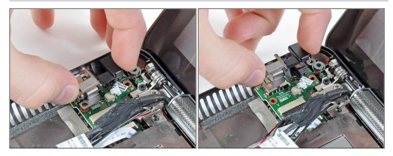
• Lift the DC jack bracket up off the USB and power board.
