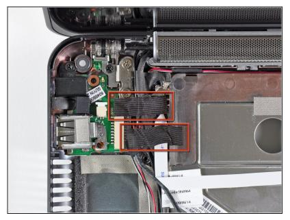
(i) If present, remove the two pieces of tape covering the cables routed near the USB and power board.
