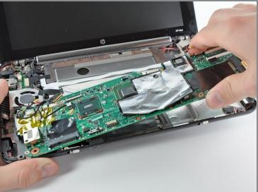
• Carefully lift the motherboard from its right edge and remove it from the lower case, minding any cables that may get caught.
