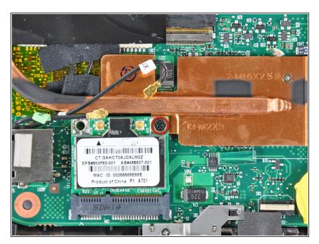
Remove the single 3 mm Phillips screw securing Wi-Fi board to the motherboard.
