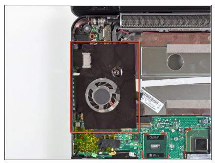
i If present, remove the large piece of black adhesive film covering the area around the fan.
