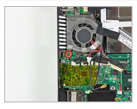
Remove the single 4.5 mm Phillips screw securing the motherboard to the lower case near the fan.
