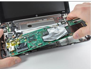
Carefully lift the motherboard from its right edge and remove it from the lower case, minding any cables that may get caught.
