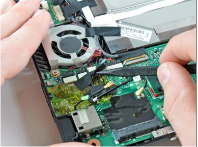
(i) If present, remove the pieces of black cloth tape securing the antenna cables to the motherboard.
