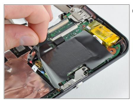
i If present, carefully peel the piece of tape covering the WWAN board.
