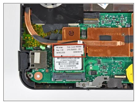
i If present, peel the sticker up off the top of the Wi-Fi board to reveal the Wi-Fi antenna connectors.
