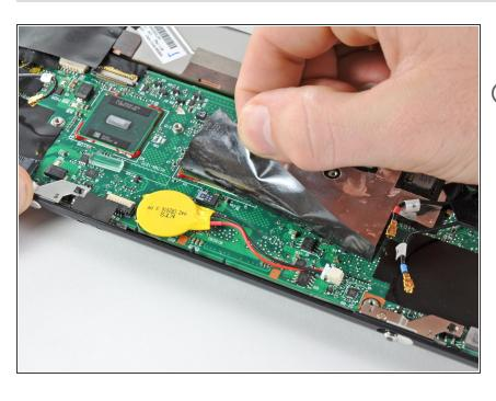
i If present, carefully peel back the piece of black film attached to the heat sink to reveal the PRAM battery and its cable.
