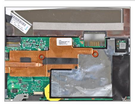
Remove the two 2.5 mm Phillips screws securing the heat sink to the motherboard.
