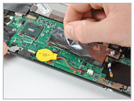
i If present, carefully peel back the piece of black film attached to the heat sink to reveal the PRAM battery and its cable.
