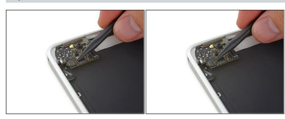
• Use a spudger to flip open the ZIF connector retaining flap for the dual microphone assembly ribbon cable.
