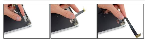
• Unfold the USB-C port ribbon cable until it lays flat, allowing access to the bracket beneath.
