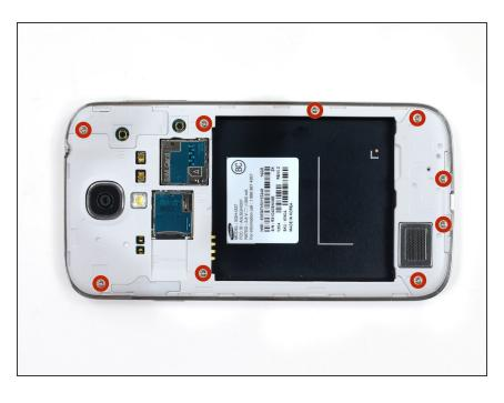
Remove the nine 4.0 mm Phillips #00 screws securing the midframe to the display assembly.
