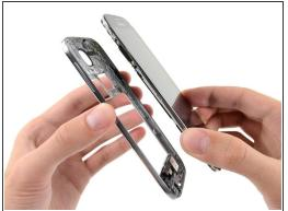
• Remove the midframe from the display assembly.
