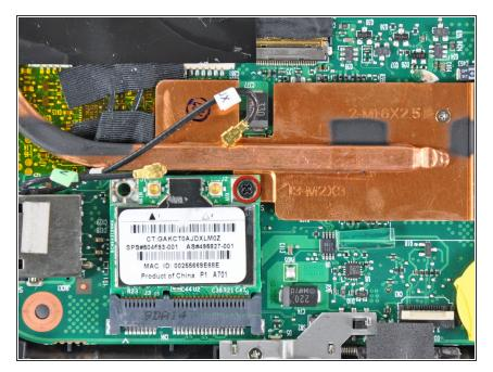
Remove the single 3 mm Phillips screw securing Wi-Fi board to the motherboard.
