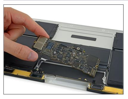
• Remove the logic board.
