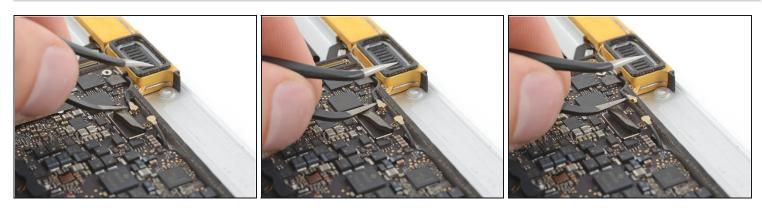
Pry up the second antenna connector to disconnect it.
