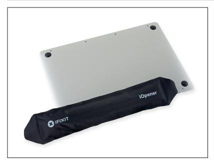
Prepare an iOpener and heat the lower case directly beneath the left speaker, in order to soften up the adhesive securing the speaker.
