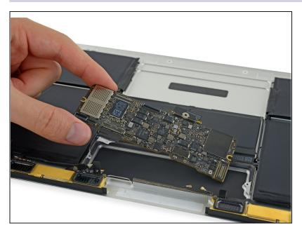
• Remove the logic board.
