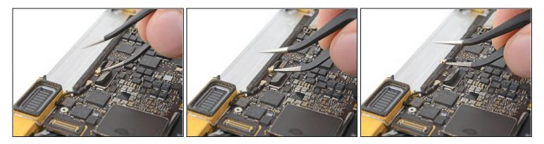
• Insert one arm of your angled tweezers under the metal neck of the first antenna connector and pry up to disconnect it.
