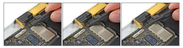
• Use the point of a spudger to flip up both ZIF connector retaining flaps.
