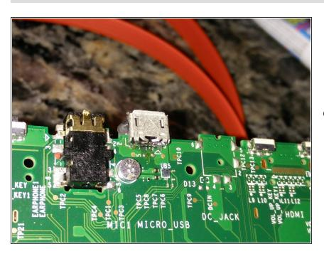
Use a multimeter or continuity tester to ensure no traces are bridged or shorted. Four of the five connector pins lead to nearby test points on the mainboard (one pin in not connected to anything). If everything works, use solder and strong epoxy to fix the new connector in place. Do not get any solder or epoxy inside the connector!
