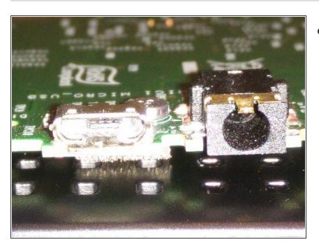
Before beginning, ensure that the USB micro jack is the problem. Try a different USB cable or charger. See if you can identify damage to the jack without opening the device. It's a bit tough to see in the photo, but this micro USB jack has been damaged: it has only four of the five internal connectors.
