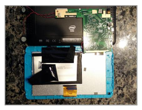
• Unscrew the three silver screws holding the mainboard in place. Flip up the plastic retainers that clamp the two ribbon cables into their connectors. Peel back any tape holding the cables or mainboard down. Then flip the mainboard over. Don't detach the wires leading to the battery or WiFi antenna! They are soldered to the mainboard.
