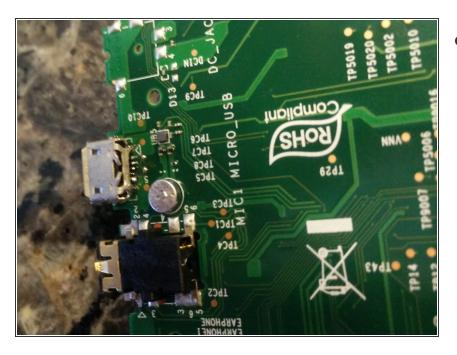
Attach the replacement micro USB connector. It helps to first clean the area with flux, and remove old solder from the traces. You'll want to gently bend the new connector's pins towards the board, and tin them and the board traces with solder in advance. Pop it into place, then heat the connector pins (not mounting posts) to secure it.
