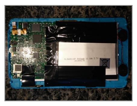
Remove the four screws that secure the back case. Gently pry off the back case, being careful not to crack
