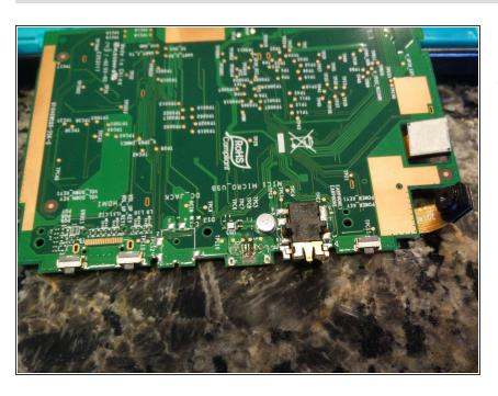
Remove the damaged micro USB connector, carefully, without damaging the mainboard or surrounding components. This is tricky. You'll want to heat it with a soldering iron, and gently pry it away from the board. You may need a helper to use pliers while you apply heat. Make sure to heat the contacts to avoid ripping the traces off the board!
