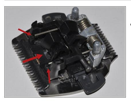
Fit the wide hair trimmer into the assembled parts.
