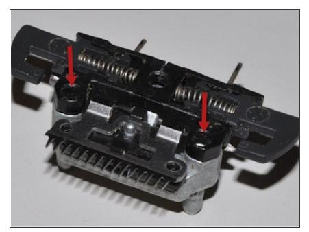
Now you can fit the locking part into the two pins (see arrows). The spring ends should not be touched here - if yes, reposition the nail.
