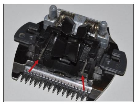
If necessary, put the spring ends behind the small guides in the wide hair trimmer part.
