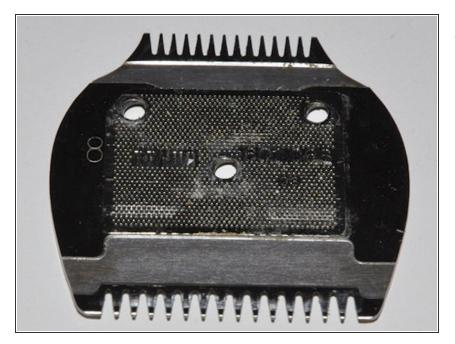
Pick the thin lubrication sheet and put it ontop of the base. Align the 3 holes.
