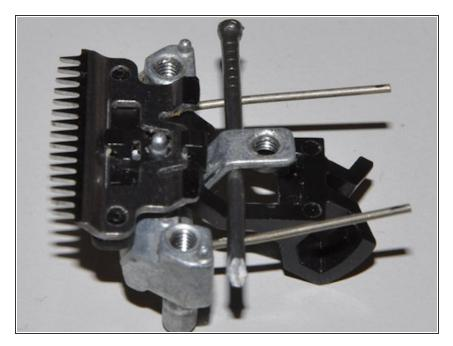
Now insert the nail in between the spring ends and the small bracket. This will hold the ends and make it possible to further assemble the head.
