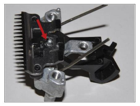
Turn around the assembled parts, and fit the short hair trimmer knives into the small pin (see arrow) of the cast piece.
