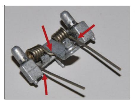
• Fit the first spring into the base (cast part). The ends have to be oriented to the bottom, as illustrated.
