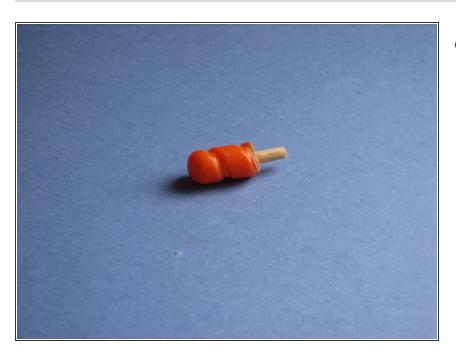
Insert the wooden dowel into one part of the broken plastic part.
