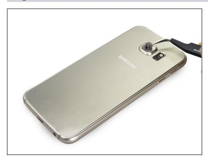
If your S6 camera lens was broken heavily, just remove it directly but very carefully.
