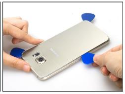
• Remove the back cover at first. It's a pity that we only have a S6 with broken back cover to show how to do camera lens glass replacement.
