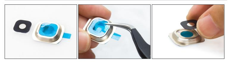
• Now it's time to place the new camera lens.Peel off the upper film and assemble the glass with the ring.
