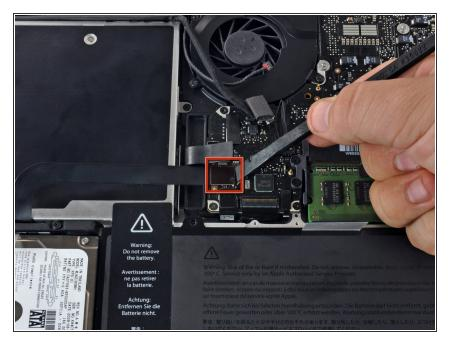
Use the flat end of a spudger to pry the hard drive connector straight up off the logic board.
