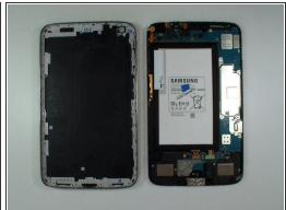
Using plastic tools remove the back / battery cover.
