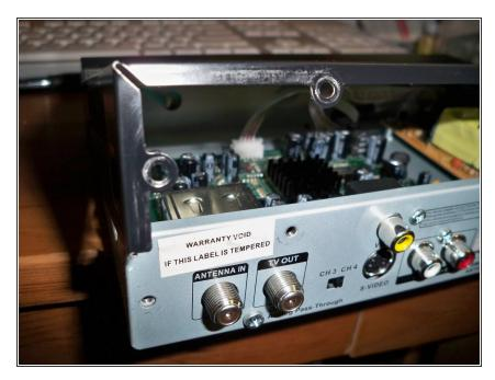
Lift the top cover up and toward you simultaneously. It shouldn't require very much force.
