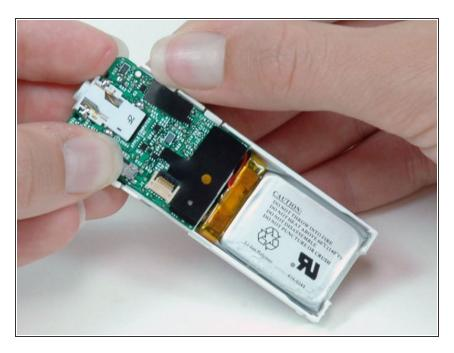
Repeat the same procedure on the opposite side to free the logic board from the white plastic casing.
