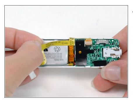
Carefully peel the yellow USB ribbon up from the battery.
