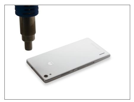
Heat to melt the adhesive sticker under the back cover.
