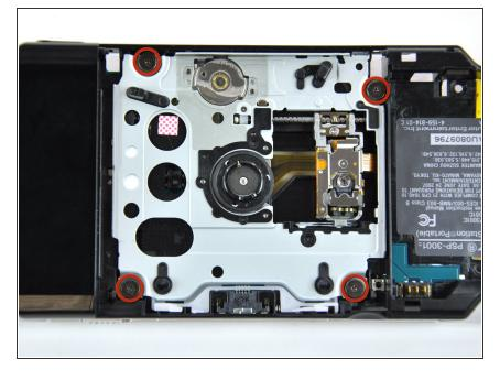
Remove the four Phillips screws securing the UMD drive to the PSP 300xc.
