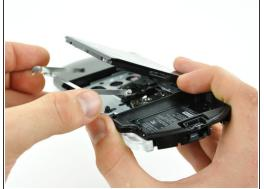
Slide the UMD brace toward the top of the UMD door until the brace disconnects from the door.
