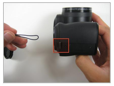
Begin by placing the string that is attached to the lens cover underneath the metal bar located on the right side of the camera.
