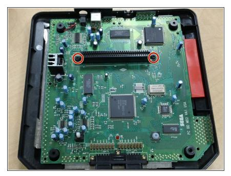
Remove the two screws highlighted in picture to remove the circuit board.
