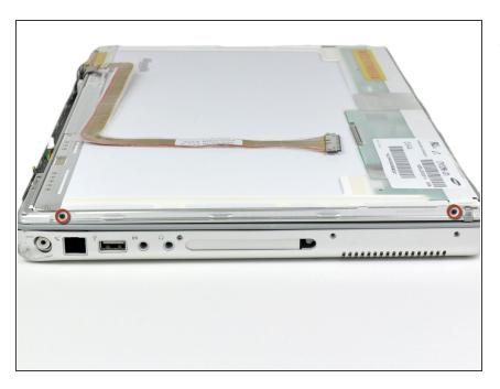
Remove the two small 3 mm black Phillips screws along DC-In side of the display.
