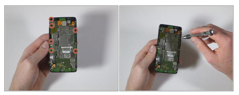
• Remove the six 4mm T5 Torx screws located along the outer edge of the motherboard.
