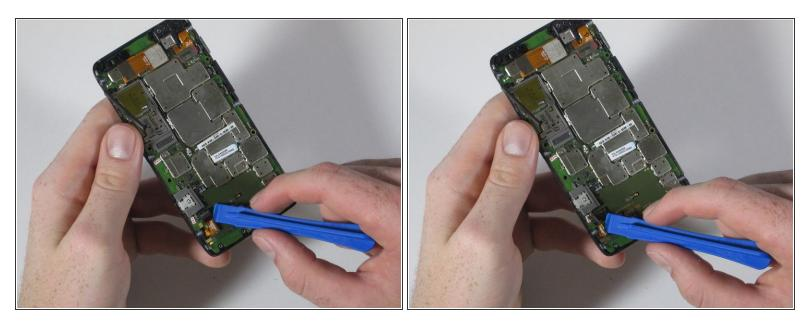
Disconnect the snap connection in the lower left corner by prying underneath using the plastic opening tool.
