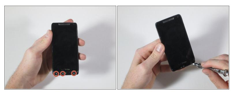
• Remove the three T4 Torx screws. There are three at the bottom of the device.
