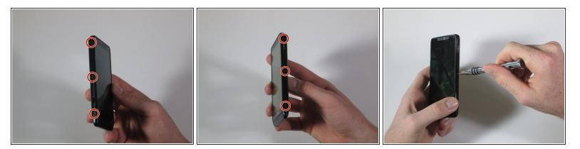
• Remove the six 4mm T3 Torx screws. There are 3 on each side of the device.
