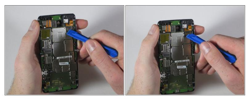
Disconnect the snap connection in the upper right corner by prying underneath using the plastic opening tool.
