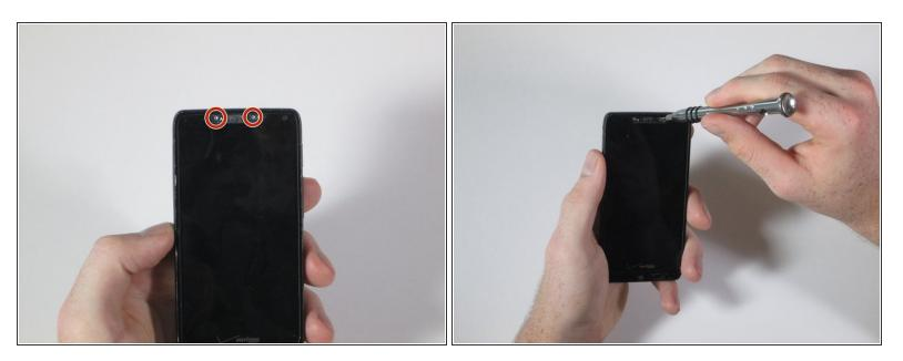
• Remove the two 7mm T4 Torx screws at the top of the device.
