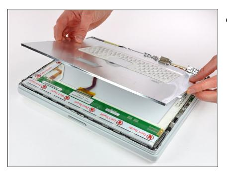
Carefully remove the thin steel LCD cover.
