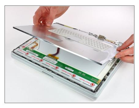
Carefully remove the thin steel LCD cover.
