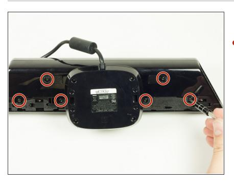
Unscrew the six 12mm T10 Torx screws.
