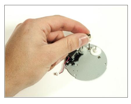
Remove the three gears on top of the motor, starting with the center gear.
