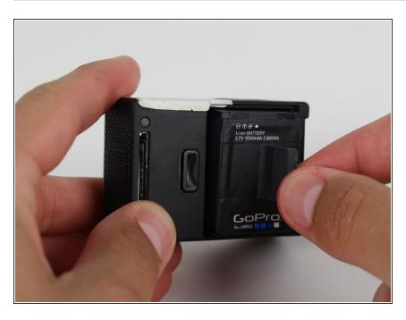
Pull the battery out using the tab.
