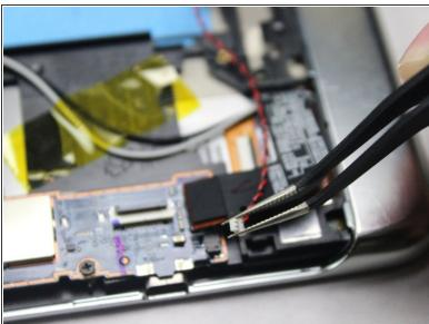
• Remove the red and black cable using the tweezers by gently pulling the connector to the right.
