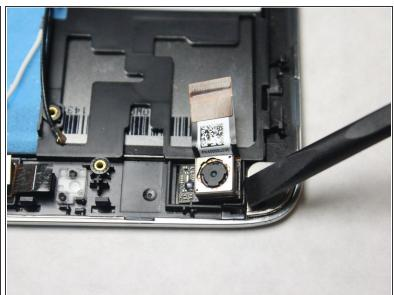
Remove the camera by carefully prying it out with the spudger.
