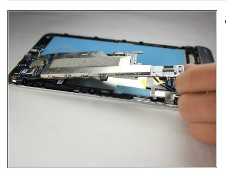
Lift the motherboard out of the tablet's case.
