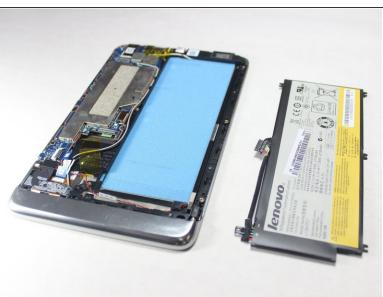
Remove the battery by prying up with your fingers or a plastic opening tool.
