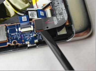
Locate the LCD cable connector and gently pry it directly up with a spudger.
