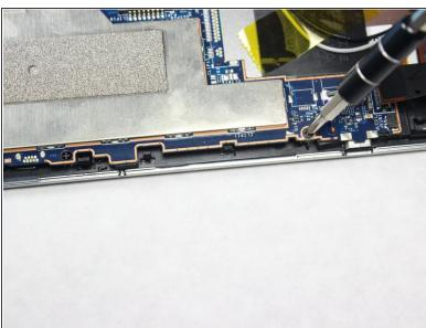
Remove the 4 1.6mm screws with a J0 head.
