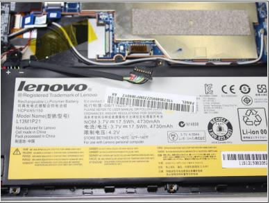
Using a plastic spudger, slowly push each side of the battery connector (back and forward a couple of times) out of its socket on the motherboard.
