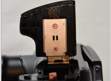
Unscrew the two 2mm screws from the inside of the case
