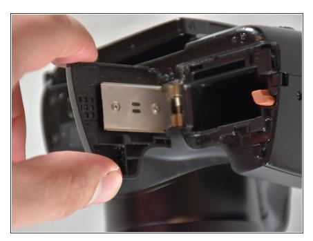
Open the protective door on the bottom of the camera, and remove the SD card and battery from the camera
