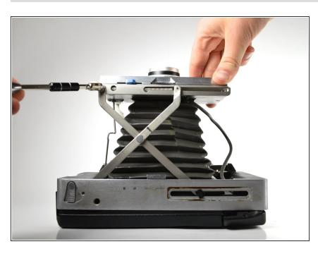
Remove the Phillips #0 6mm screw on the shutter mount and the washers using a size 5 nut driver.
