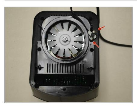
Remove these two screws (10mm long, 5mm head diameter) using a Phillips #2 screwdriver.
