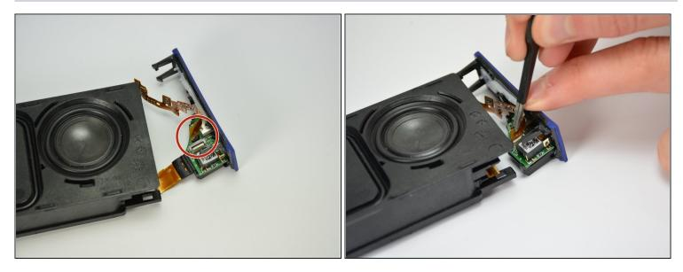
• Reconnect the button ribbon connector on the top of the port assembly.
