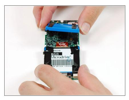
• Lift the battery off of the logic board and lay it to the side of the iPod.
