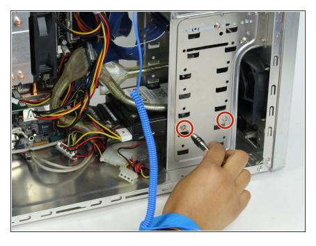
Remove two Phillips #2 head 5mm screws holding the hard drive in place.
