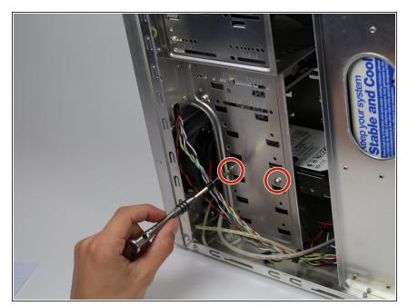
Remove two Phillips #2 head 5mm screws holding in the other side of the hard drive.
