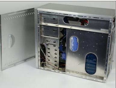
Next, remove the side panel of the computer case to allow access into the computer.
