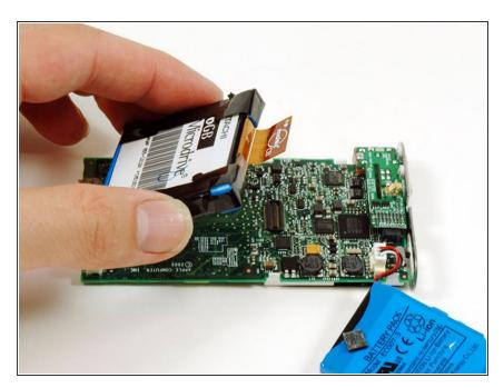
• Lift the hard drive out of the iPod.
