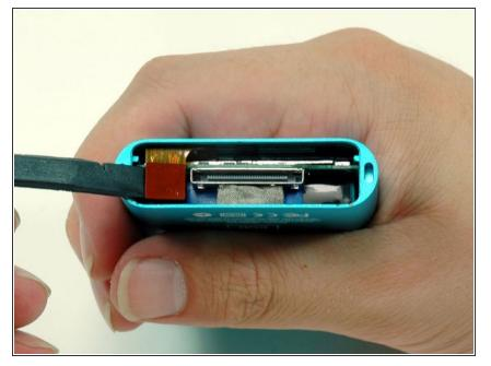
Use a spudger or the tip of your finger to carefully disconnect the orange click wheel ribbon from the logic board.
