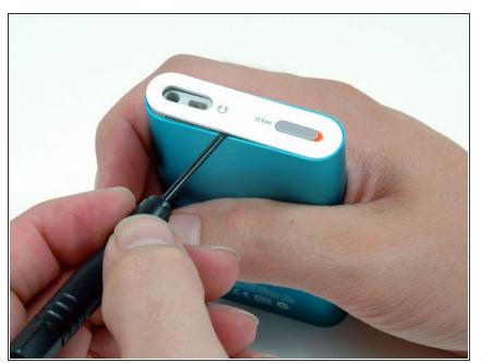
• Carefully insert a small flathead screwdriver or <u>Jimmy</u> in the seam between the metal casing and white plastic top. Use the screwdriver to pry up the white plastic top bezel. Be careful not to damage the soft plastic with your screwdriver.
