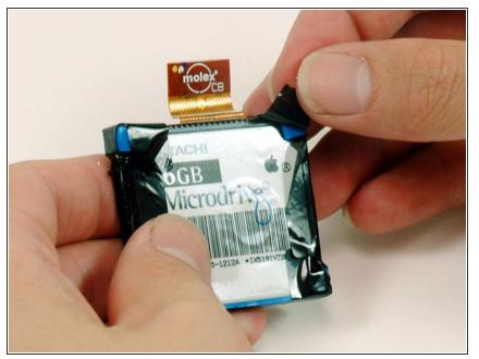
• Peel back the black tape securing the two blue bumpers to the hard drive near the orange ribbon cable.
