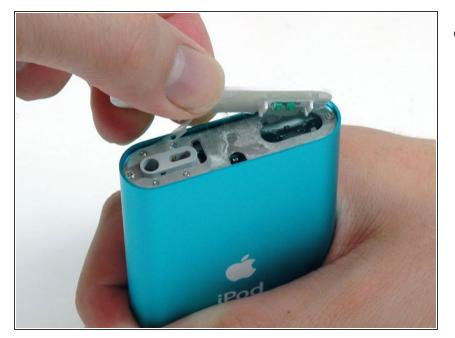
• Lift the top bezel off of the iPod.
