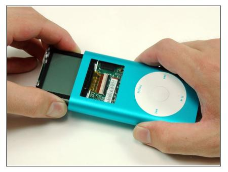
After pushing the logic board out sufficiently, gently grasp the logic board on either side of the display, and continue to slide the iPod out of its casing.
