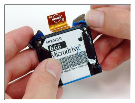
• Slide the two blue bumpers off the corners of the hard drive. There is no need to remove these bumpers entirely.
