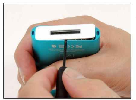
Carefully insert a small flathead screwdriver or <u>Jimmy</u> in the seam between the metal casing and white plastic bottom Use the screwdriver to pry up the white plastic bottom bezel. Be careful not to damage the soft plastic with your screwdriver.
