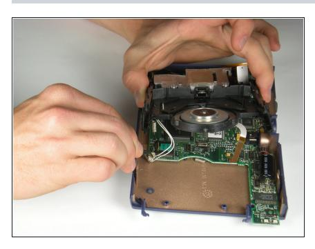
Disconnect the white wires by using tweezers to gently pull the bottom connector toward you.
