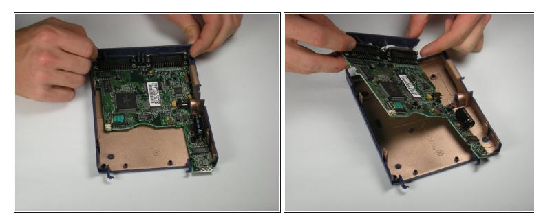
• Gently lift the motherboard and back case out from the bottom case.
