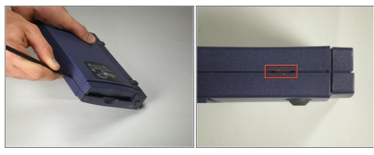
• Push in the plastic tab that can be seen through cracks in the front left corner using a spudger.
