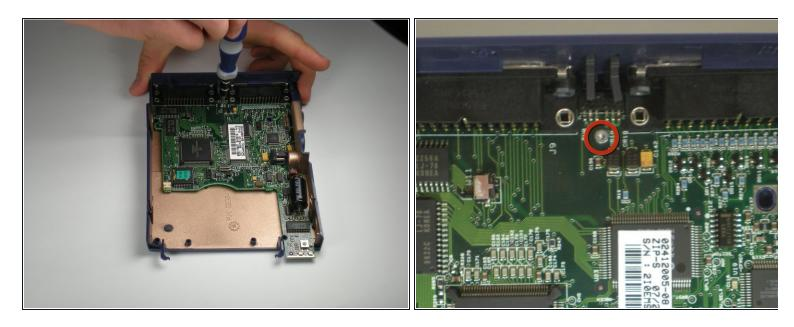
• Use a T6 Torx Screwdriver to remove the 1.3 mm screw at the back of the motherboard.
