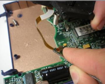
Disconnect the thin ribbon wire by using tweezers to gently pull the connector at the bottom toward you.
