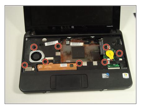
• Remove the eight screws that are from the plastic top cover.
