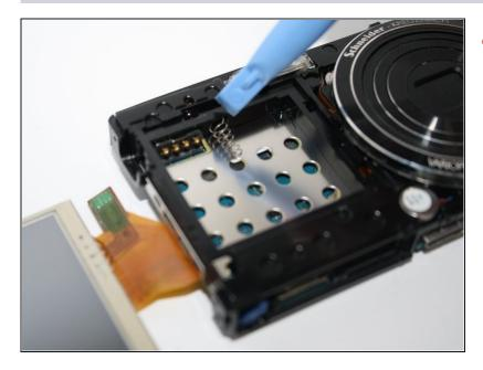
After all the parts are disassembled, you will reach the spring part of the camera.
