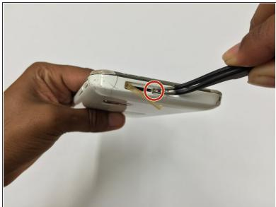
Remove the SD Memory Card before taking the device apart. Using the screwdriver, remove the 10mm Phillips screw that is near the SD Memory Card port.
