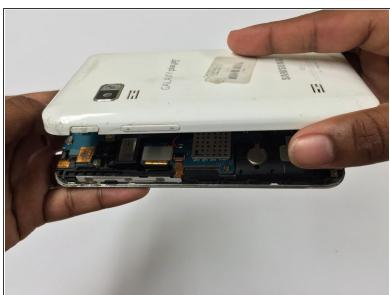
Take the back housing cover off of the device.
