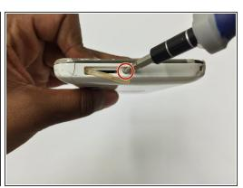
Lastly reinsert the screws at the bottom of the device, as well as the screw inside the SD Memory Card port.
