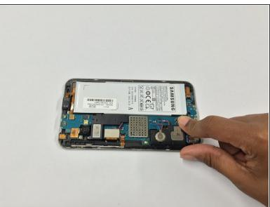
Insert the battery into its position, and reconnect its tab onto the motherboard.
