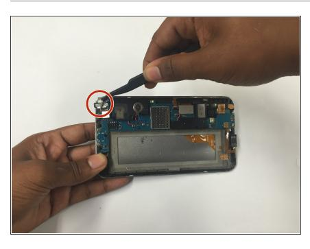
Place new the headphone jack back into its position and connect the tab, then screw it back into place.
