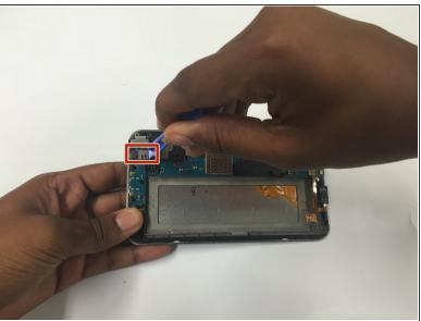
• Remove the headphone jack by unscrewing the 10mm Phillips screw to its left then proceed to pry up the tab that attaches the headphone jack to the motherboard.
