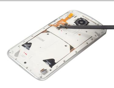
Use the flat end of a spudger to gently pry up the ribbon cable in the two places where it is adhered to the battery.
