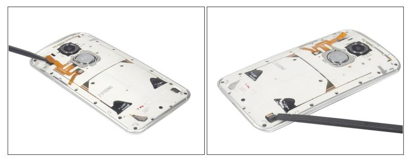
Use the spudger to release the connectors from under the covers.
