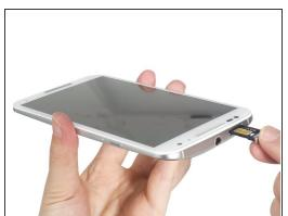
Remove the SIM card tray by inserting the SIM card eject tool into the small hole on the tray.
