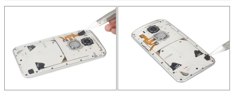
Remove the rubber covers from the two connector pieces indicated in the photo
