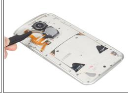
Remove the logo, as the flex cable under the logo is fastened to the back of the battery. This can be done by removing the three surrounding screws, and then prying off the structure that encapsulates the logo.
