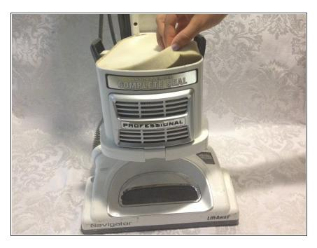
At the base of the vacuum will be a large plush filter. This is one of two filters in this compartment. Take this filter out.
