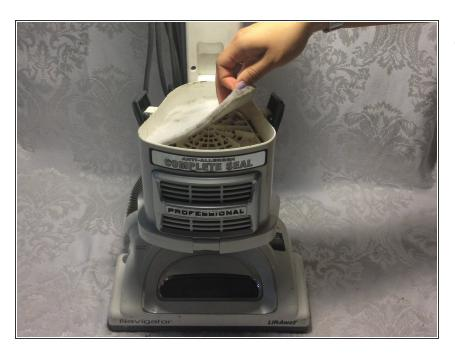
The second filter is thinner and lies at the base of the vacuum. Replace this filter first before placing the larger replacement filter on top of it.
