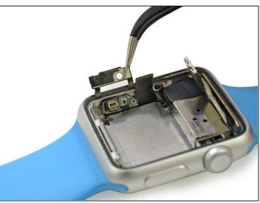
• Given the limited amount of <u>space</u> inside the Apple Watch, we find the microphone ribbon cable creatively ensnared between the inner and outer layers of the case.
