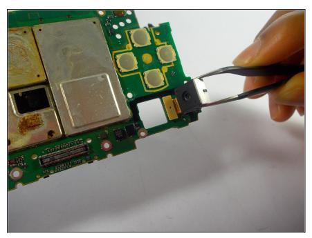
With the camera facing away, pull it from the motherboard until it stands perpendicular to the board. <u>Tweezers</u> can be used to do this.
